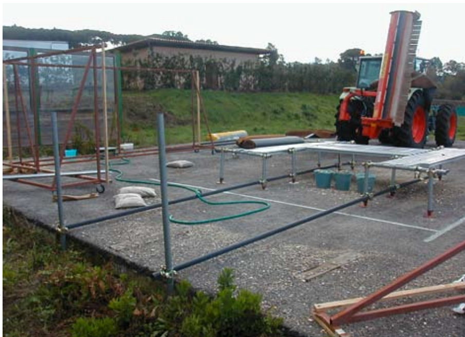
Test site preparation for stone ejection testing of highway maintenance and agricultural machines and implements.
